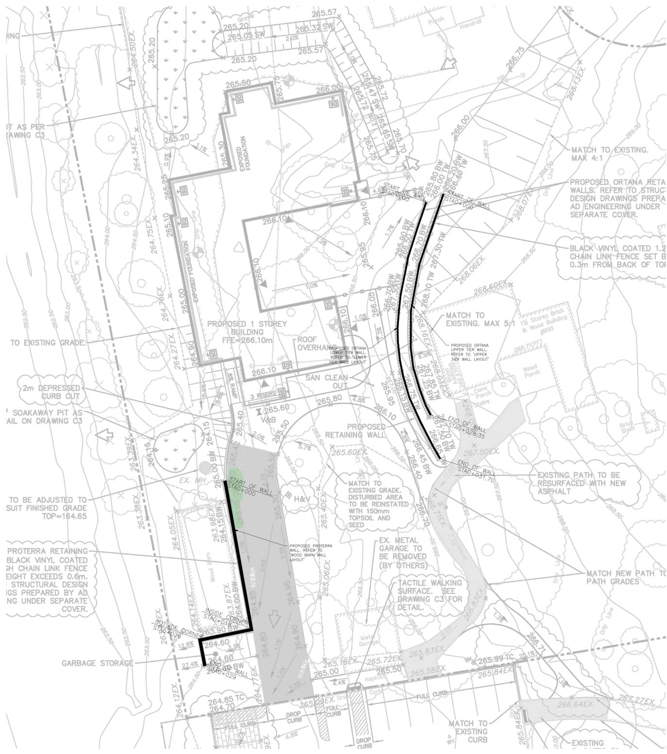
PROPOSED RETAINING WALL PLAN SCALE: 1:200
