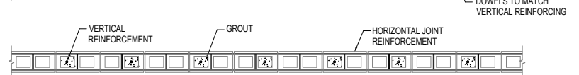
WALL TYPE (2) (20MPa BLOCKS) TYPICAL 290 MASONRY BLOCK SHEAR WALL (PERPENDICULAR TO JOISTS) SCALE: NOT TO SCALE
