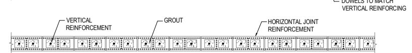
WALL TYPE (1) (20MPa BLOCKS) TYPICAL 290 MASONRY BLOCK SHEAR WALL (PARALLEL TO JOISTS) SCALE: NOT TO SCALE
